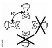
Figure 1. Acceptable Outdoor Mounting Positions with Weather Shield.
