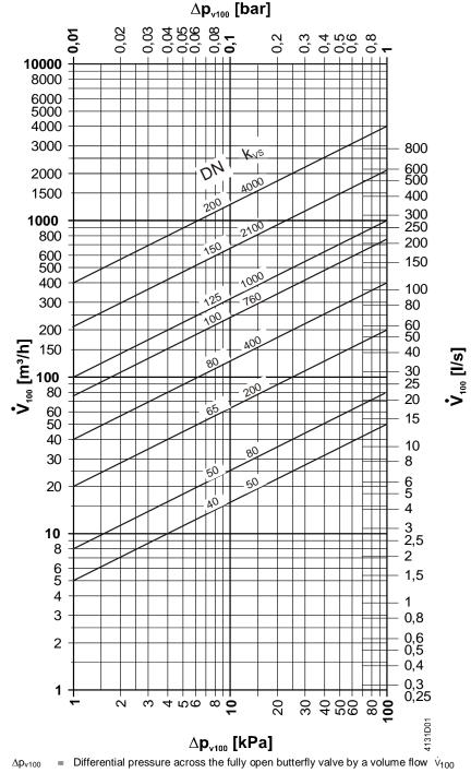
$\dot{V}_{100}$  = Volume flow through the fully open butterfly valve
