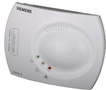
**Electronic gas leak detectors with one threshold for residential use. 230VAC power supply, SPDT relay output suitable for 230VAC solenoid valve or other signalling or activating devices.**
