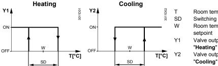
Room temperature Switching differential Room temperature setpoint Valve output signal "Heating" Valve output signal
