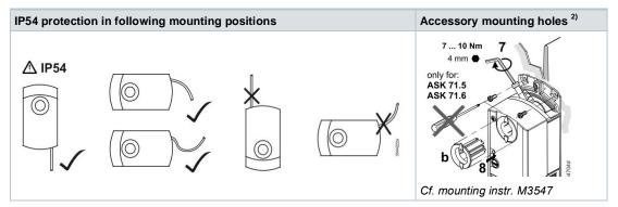
$oldsymbol{\Lambda}$   $^{2)}$ Not to be used for fixation of the actuator, use anti-rotation-bracket instead.
